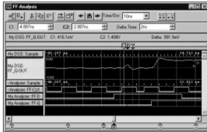
Figure 2–13: Using the DSO module to capture a runt pulse
